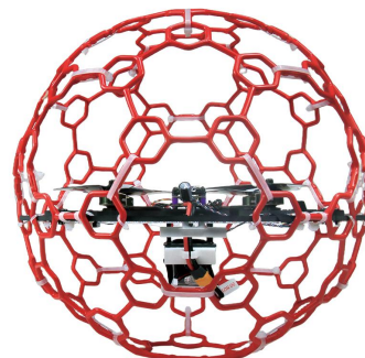
Pitch stick upward, LDZ-A40 moves forward
