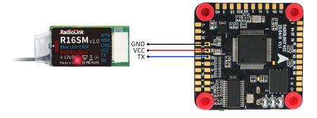
Please set SERIAL1\_PROTOCOL to 2 in Mission Planner. (Depend on the used serial port ) And please select CC2500 on the telemetry information menu of T16D/T12D:
