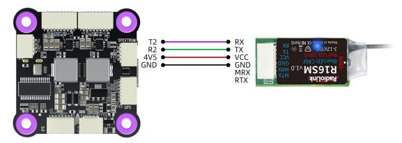
Please set parameters in Betaflight/INAV configurator. Here are the setting steps. Click Ports and open the used serial port. Click Receiver. Select Serial (via UART)--Select CRSF--Turn on Telemetry--Click Save. The steps are as shown below:
