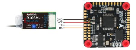
Please set SERIAL1\_PROTOCOL to 2 in Mission Planner. (Depend on the used serial port ) And please select RX CRSF on the telemetry information menu of T16D/T12D:
