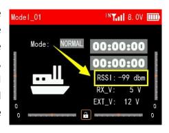
(2) Make the receiver antenna and transmitter antenna parallel. Keep transmitter apart from receiver about 60 centimeters and both antennas straight. It is normal that RSSI value is within the range of 0 to -30dBm. The closer the value is to 0, the stronger the signal is.
