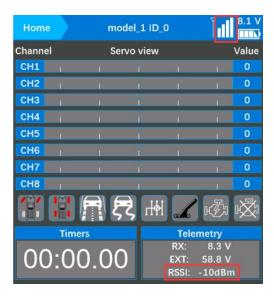
Warning can be set with a certain low RSSI value after testing by changing distance. Enter Telemetry setting--Receiver signal to set the RSSI warning value, alarm sound type etc.
