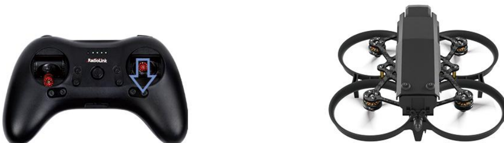
Pitch stick downward, F108 moves backward
