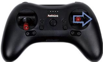
Roll stick to right, F108 fly to the right side
