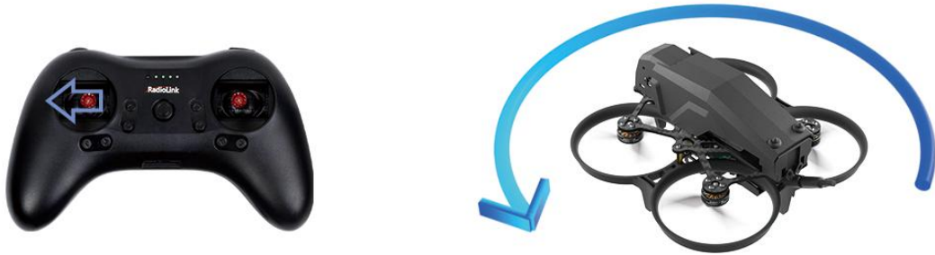
Yaw stick to the left, F108 turns anticlockwise
