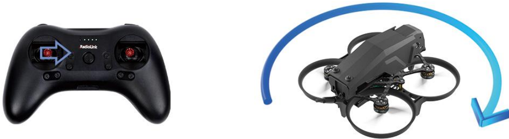
Yaw stick to the right, F108 turns clockwise
