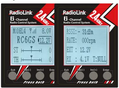
Warning can be set with a certain low RSSI value after testing by changing distance: Press EXIT and ENTER simultaneously to enter MENU=>press Inc(+) to highlight "19. ALARM =>Press ENTER to (dis)activate the warning and set the RSSI warning value.
