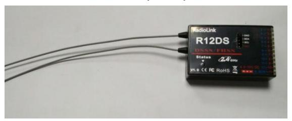
Radiolink R12DS, 2.4G 12 channels receiver, DSSS and FHSS spread spectrum working synchronously, compatible with Radiolink transmitters AT9, AT9S, AT10 and AT10II(AT9, AT9S, AT10 can upgrade to 12 channels just upgrade by firmware, you can download the firmware from our website: http://radiolink.com.cn/doce/at10upgraded.html , AT10II is default 12 channels).
