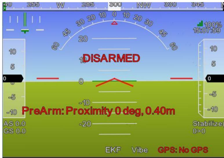
The above screenshot shows SUI04 detects the distance less than 60cm and is locked by the flight controller. To armed SUI04, the distance between the drone and obstacles should be more than 60cm.
