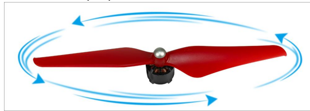
CCW propellers (counterclockwise rotation)
